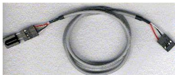
Sensor - 2-wire + ground cable - To infrared connector
