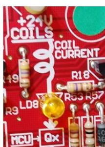
This coil current is displayed on the **PI-1 X4** board by an additional « **COIL CURRENT** » status LED. In case of trouble, the **PI-1 X4** board displays a specific error message along with the problem source, and if needed, the coil protection relay **RLY1** and its status LED are turned off to shut all coils down and avoid further damage.
