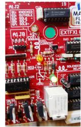
The LED on the center right of the board, with the electrical symbol of a coil (*spiral*), shows that the coil protection relay **RLY1** is on and that power is fed to the playfield coils. It should be normally unlit, and lit during a game.
