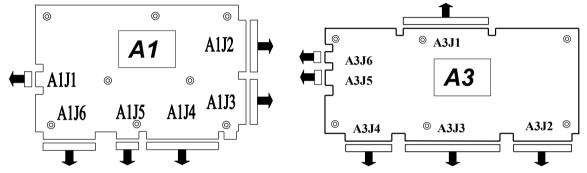
Write down the way they are inserted, then remove them following the arrows above: pull on the **plastic case**, and **not on the wires!** The wire harness between **A1J4** and **A3J1** is no longer used.
