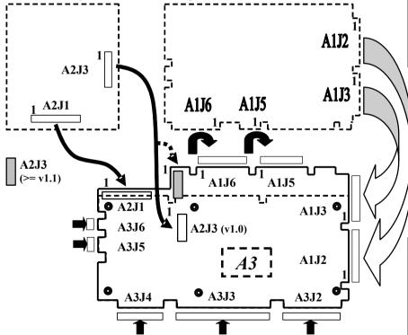
There is no possible risk of mistake or confusion of the connectors: each connector has its own specific size, and some have notches (blockers), making mix-ups impossible.
