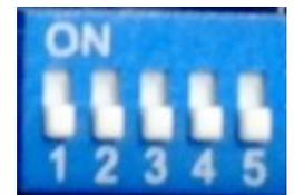
By default, the **PI-FX/X4** board is delivered in « **AUTO** » configuration (DIPSW **S1/S2/S3** = OFF) : the main **PI-1 X4** board configures the **PI-FX/X4** board automatically upon power-up if the game is among this list: **Totem, Hulk, Genie, Buck Rogers, Torch, Roller Disco, Asteroid Annie**. It is always possible to change that game setting manually, even while the game is on, by means of DIPSW **S1/S2/S3**.
